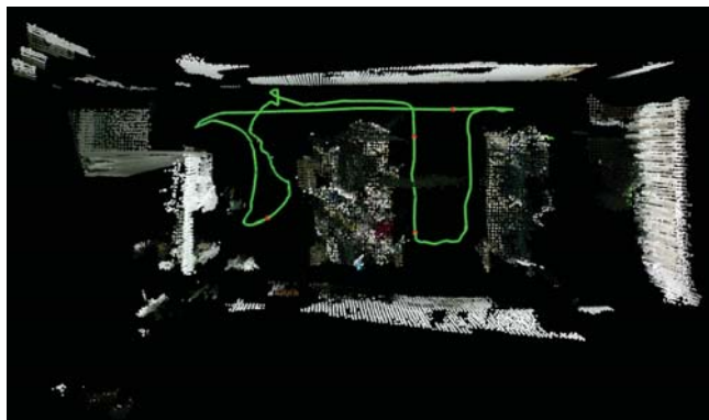
Fig. 7 Re-localization in the office dataset. Green points are the correct re-localization, while red points are the incorrect matching
