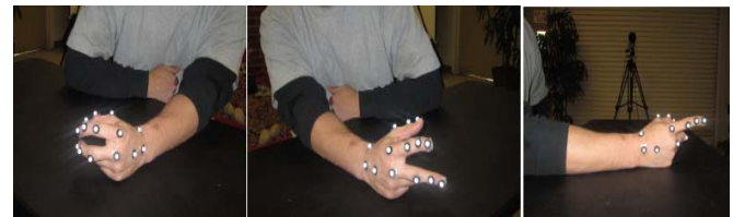
Fig. 6 Marker set up for extracting motion capture data from the three main training motions: pinch, palm open/close and point
