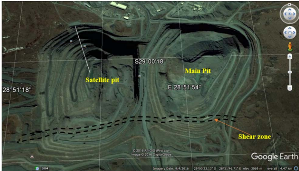
Fig. 1 Shear Zone Across Satellite and Main Pits at Letšeng Diamonds Mine in Lesotho
