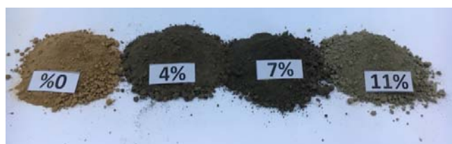
Fig. 2 Dredged materials with different OMCs
