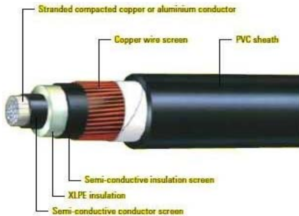
Fig. 17 Cross-sectional area for the 11KV cable
