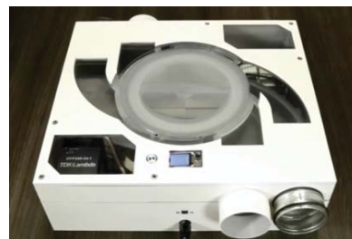
Fig. 4 Laboratory prototype of the Counterflow Heat Recovery Fan (CHRF) [2]
