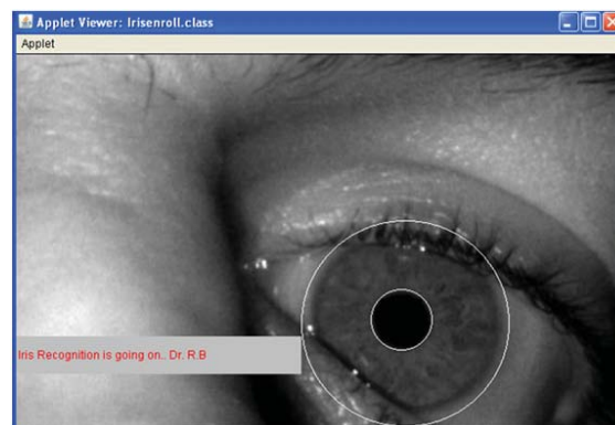
Fig. 5 Illustration of Outer boundary detection and Occlusion of eyelashes/eyelids on the iris
