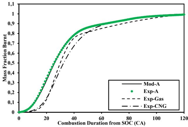
Fig. 8 (a) Comparison of Experimental and dual Wiebe modeled curves of PG Set-A operation at WOT,  $\Phi=1.09$ , rpm=1500 and modeled coefficients  $x=0.82$ ,  $a_1=52$ ,  $m_1=1.43$ ,  $a_2=6$ ,  $m_2=2$
