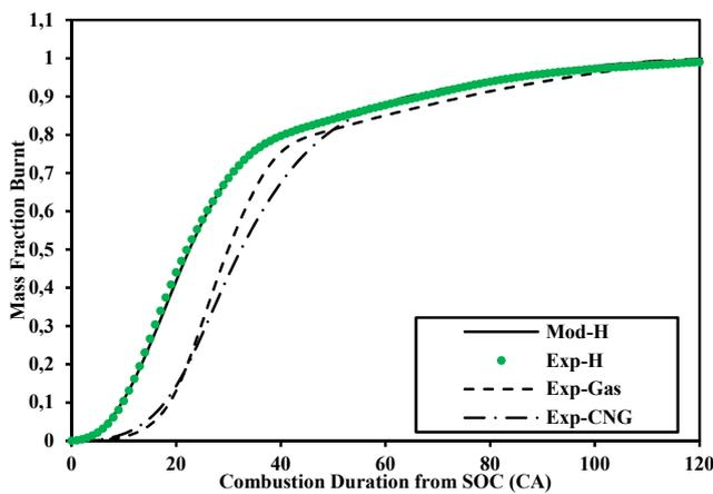
Fig. 8 (h) Comparison of Experimental and dual Wiebe modeled curves of PG Set-H operation at WOT,  $\Phi=1.18$ , rpm=1500 and modeled coefficients  $x=0.783$ ,  $a_1=70$ ,  $m_1=1.35$ ,  $a_2=5.7$ ,  $m_2=1.8$
