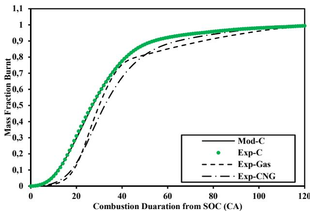
Fig. 8 (c) Comparison of Experimental and dual Wiebe modeled curves of PG Set-C operation at WOT,  $\Phi=0.94$ , rpm=1500 and modeled coefficients  $x=0.86$ ,  $a_1=35$ ,  $m_1=1.35$ ,  $a_2=5$ ,  $m_2=1.75$
