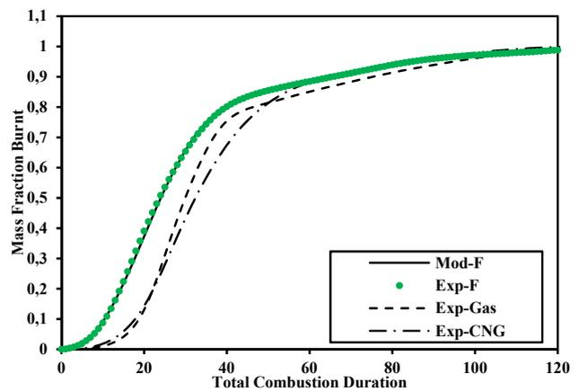
Fig. 8 (f) Comparison of Experimental and dual Wiebe modeled curves of PG Set-F operation at WOT,  $\Phi=1.16$ , rpm=1500 and modeled coefficients  $x=0.82$ ,  $a_1=66$ ,  $m_1=1.35$ ,  $a_2=6$ ,  $m_2=1.85$
