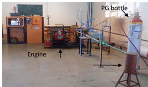
Fig. 1 PG experimental set-up
