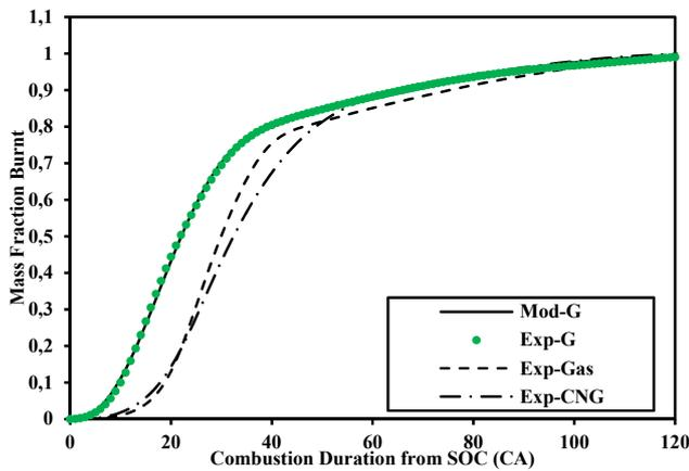
Fig. 8 (g) Comparison of Experimental and dual Wiebe modeled curves of PG Set-G operation at WOT,  $\Phi=1.15$ , rpm=1500 and modeled coefficients  $x=0.785$ ,  $a_1=75$ ,  $m_1=1.38$ ,  $a_2=5$ ,  $m_2=1.7$
