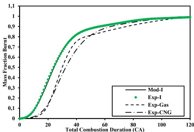
Fig. 8 (i) Comparison of Experimental and dual Wiebe modeled curves of PG Set-I operation at WOT,  $\Phi=0.97$ , rpm=1500 and modeled coefficients  $x=0.84$ ,  $a_1=65$ ,  $m_1=1.45$ ,  $a_2=6$ ,  $m_2=1.8$
