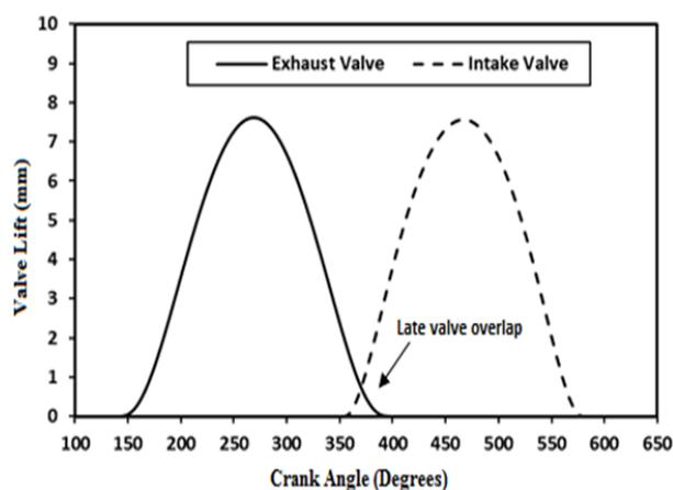
Fig. 5 Unsymmetrical negative valve overlap for specified engine
