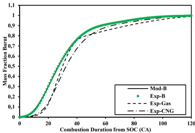
Fig. 8 (b) Comparison of Experimental and dual Wiebe modeled curves of PG Set-B operation at WOT,  $\Phi=1.06$ , rpm=1500 and modeled coefficients  $x=0.85$ ,  $a_1=30$ ,  $m_1=1.31$ ,  $a_2=5$ ,  $m_2=2$
