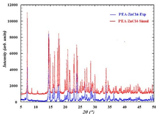
Fig. 1 Experimental and simulated X-Ray diffraction patterns of PEA-ZnCl<sub>4</sub>
