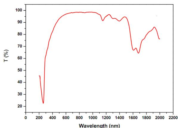
Fig. 4 UV-visible transmittance spectrum of PEA- $\text{ZnCl}_4$
