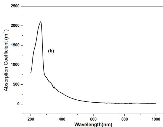
Fig. 5 Optical absorption coefficient ( $\alpha$ ) for PEA-ZnCl<sub>4</sub>
