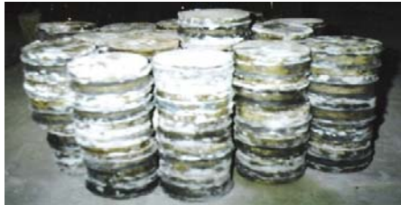
Fig. 8 Specimens subjected to chloride penetration
