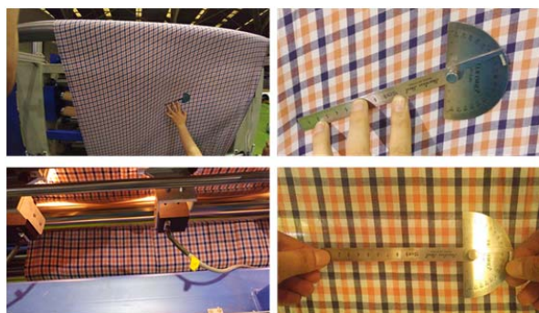
Fig. 13 Comparison of before and after controlling weft straightener (skew angle)
