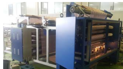
Fig. 12 Weft straightener and simulator test configuration
