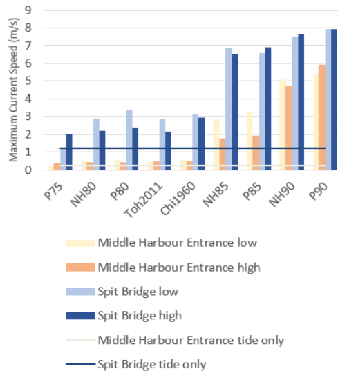
Fig. 6 Maximum current speeds for the high/low series at locations Spit Bridge and Middle Harbour Entrance
