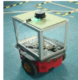
Fig. 6 Mobile robot (Pioneer 3DX) and RPLIDAR (black disc on top) as part of the N-MARIA structure
