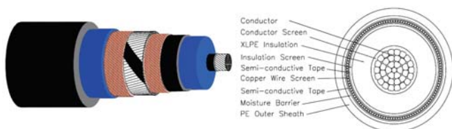
Fig. 3 Single core submarine power cable cross section [3]
