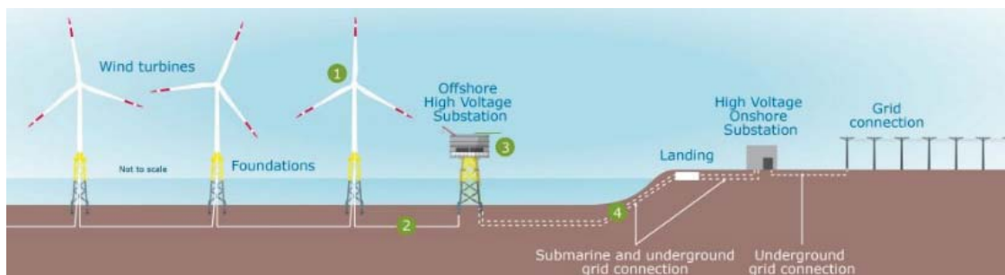
Fig. 1 Offshore wind farm main components [1]
