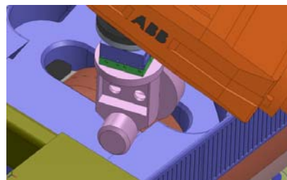
Fig. 8 UFC Grinding (or Milling)- using Robot “B”
