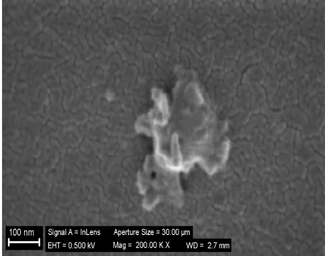
Fig. 5 Magnified SEM images of pristine PVDF/GO, displaying details of the GO sheets
