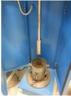
Fig. 5 CBR mould with sediments ready to be compacted with the tamper
