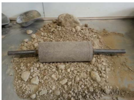
Fig. 4 Grinding the sediments after oven drying
