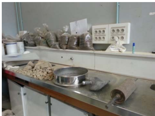
Fig. 3 Material for grinding and sieving dry sediments (from left to right: a 20 mm sieve, a knife and a roller)
