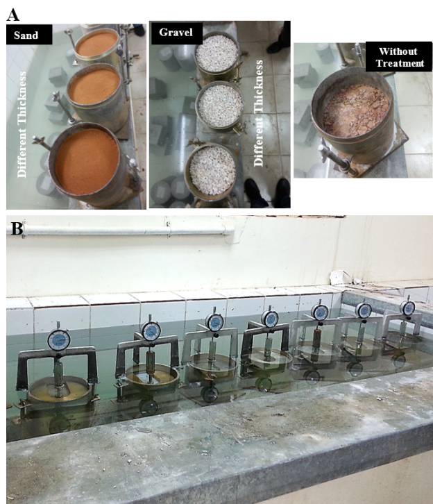
Fig. 6 Seven undisturbed shale molds (6 treatments and 1 without) with different type and thickness of replacement CCS used for treatment (A); seven molds submerged in a water tank and fixed a dial gage (0.01mm) for measurement of swelling (B); Al Qadsiyah district, Tabuk, KSA
