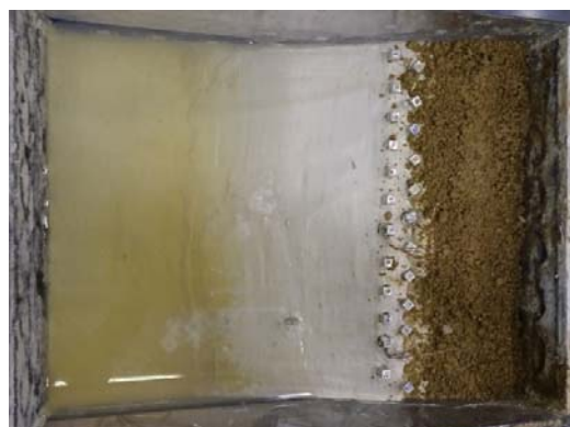
Fig. 5 Top view of piles group box
