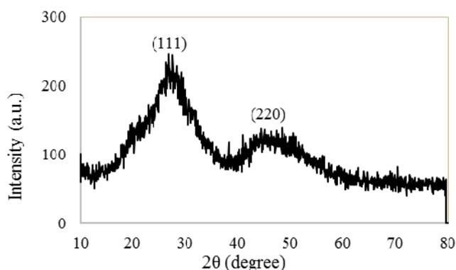
Fig. 2 The XRD pattern of biosynthesized CdS nanoparticles
