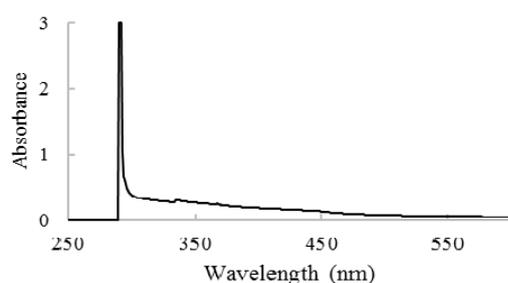
Fig. 6 UV-Vis spectra of biosynthesized CdS nanoparticles
