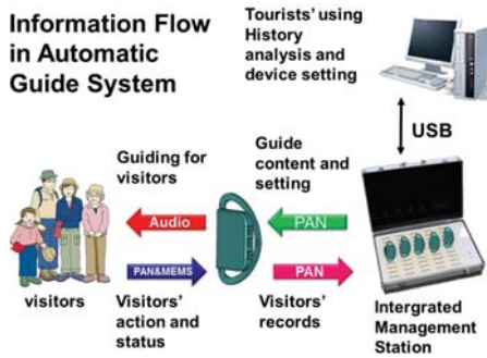
Fig. 7 The total information flow in the guidance system
