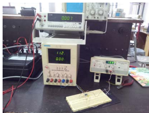
Fig. 5 Experimental setup for one amplifier loop test method
