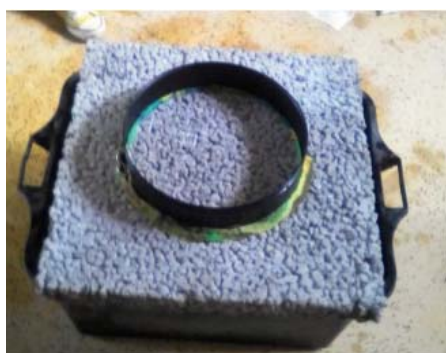
Fig. 3 Pervious concrete permeability test setup [13]
