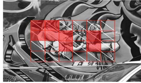
Fig. 4 Patch Grids for Image Alignment, eight patches with the highest intensity gradient are highlighted and used in the ESM optimization
