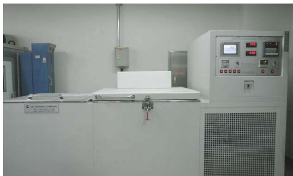
Fig. 4 Freezing-Thawing Resistance Measurement Equipment
