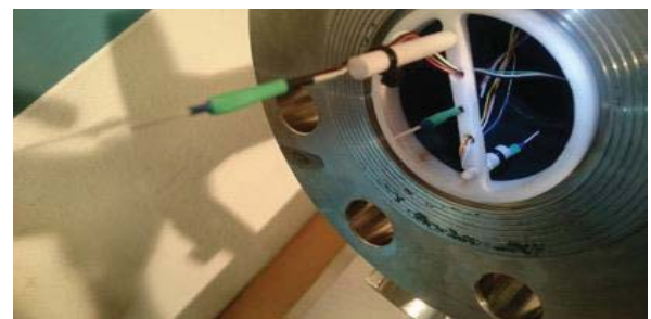
Fig. 10 Internal view of the opened ‘Supercritical Chamber’. Three temperature sensors are attached to a white Teflon structure which a negligible thermal conductivity. These sensors are used to monitor the temperatures inside the gas
