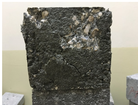
Fig. 3 Specimen after compressive strength test
