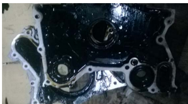
Fig. 4 Contaminates and sludge accumulated in the oil pump
