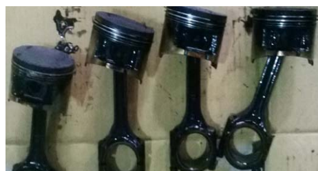
Fig. 8 Disassembled pistons and connecting rods
