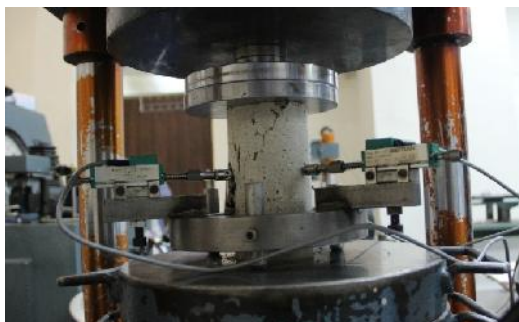
Fig. 3 Uniaxial compression test setup
