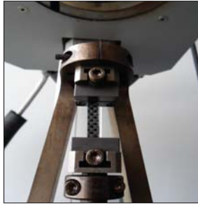
Fig. 1 Configuration of a segment of the facesheet traction test in the TMA device
