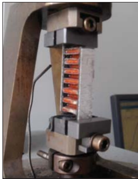
Fig. 2 Configuration of a segment of the core shear deformation in the TMA device
