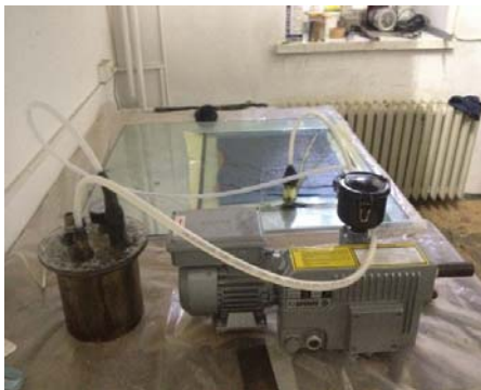
Fig. 1 Vacuum bagging system set-up
