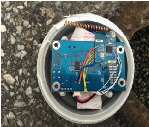
Fig. 5 The sensor node in enclosure
