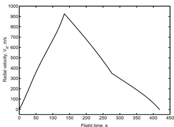
Fig. 7 Radial velocity variation over Zenit-2 flight time
