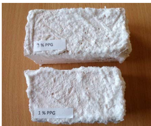
Fig. 7 Geopolymer mortar specimens containing 1 and 2% of PPG
