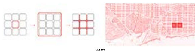
Fig. 1 1859 Example block, new Superblock three-by-block area with periphery streets, and Superilla interior pedestrianized streets of limited vehicular traffic
