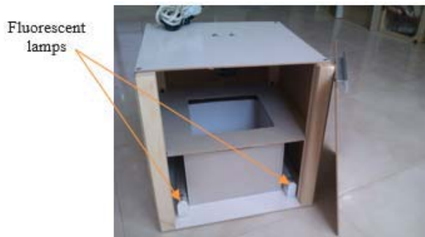
Fig. 1 Imaging chamber and the position of fluorescent lighting
