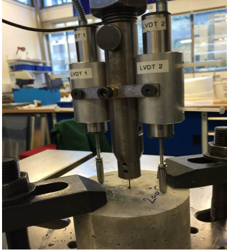
Fig. 2 Single fibre pull-out test setup
