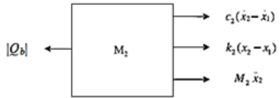
Fig. 4 Magnitude of Dynamic Earth Thrust
