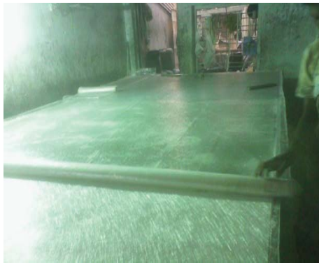
Fig. 2 Hand Laying Process
