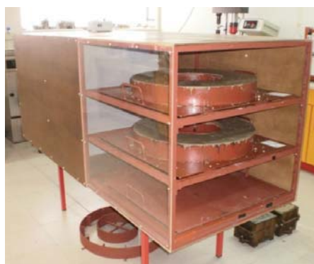
Fig. 2 Cracking specimens in the wind tunnel
