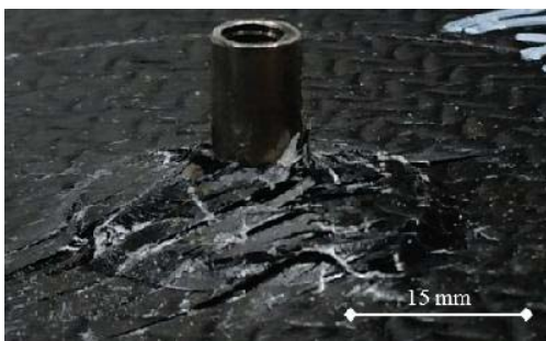
Fig. 8 Post-mortem picture of a specimen tested with 150 mm/min
