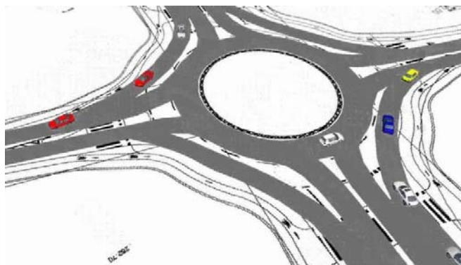
Fig. 9 Typical flower roundabout (showing segregated right-turn)
