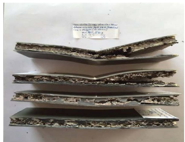
Fig. 9 Collapsed sandwiches named S1.75A after the bending tests at different support span values (top to bottom: L = 55, 70, 80 and 125 mm)
