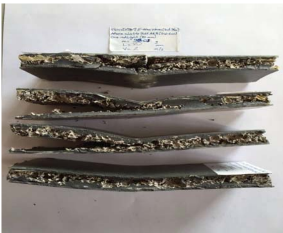
Fig. 7 Collapsed sandwiches named E1.75A after the bending tests at different support span values (top to bottom: L = 55, 70, 80 and 125 mm)
