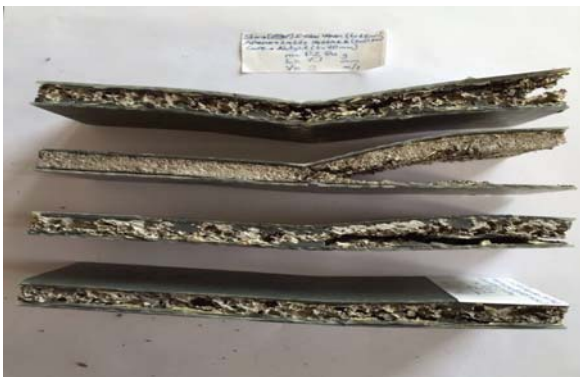
Fig. 6 Collapsed sandwiches named E1.5A after the bending tests at different support span values (top to bottom: L = 55, 70, 80 and 125 mm)
