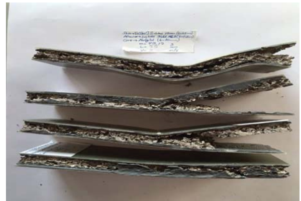
Fig. 8 Collapsed sandwiches named S1.5A after the bending tests at different support span values (top to bottom: L = 55, 70, 80 and 125 mm)
