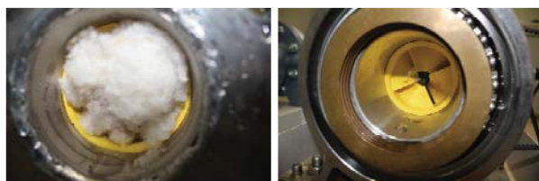
Fig. 11 Guide vane and runner of D_2/D_1=0.25
