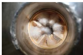
Fig. 9 Guide vane of D_2/D_1=0.375
