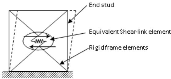
Fig. 2 Illustration of the shear wall model
