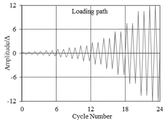
Fig. 5 CUREE reversed cyclic test protocol
