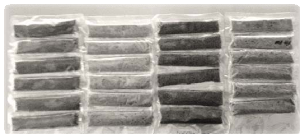
Fig. 2 Pulse spreads after high pressure processing in flexible transparent PA/PE packaging material pouches
