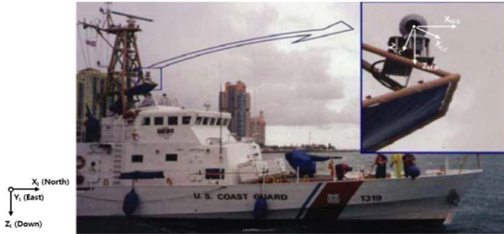
Fig. 1 Schematics of the coordinate frames (Example: USCG Thetis [8])
