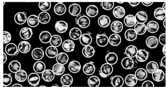
Fig. 5 Detail of the resulting image with highlighted circles representing edges of fibers
