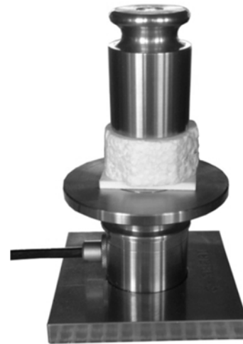
Fig. 11 Measurement of the thermal conductivity with TCi C-Therm
