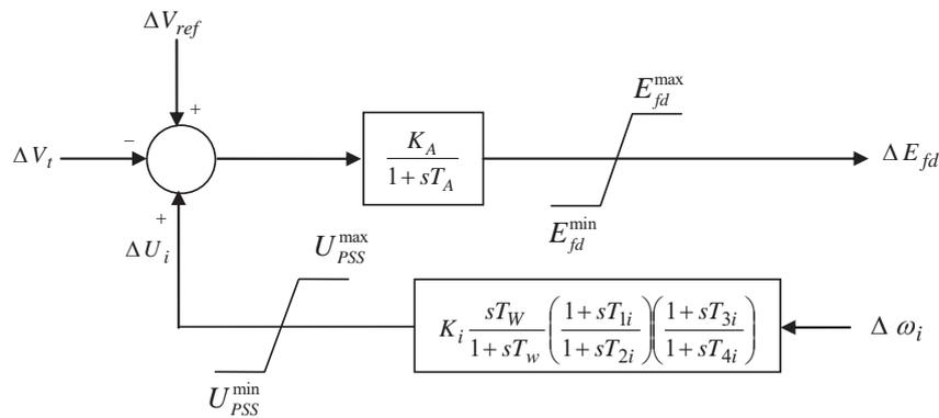
Fig. 2 IEEE Type-ST1 excitation system with PSS
